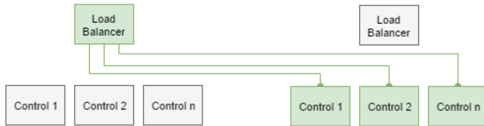
Figure 6. Instances on the load balancer are replaced with new ones
